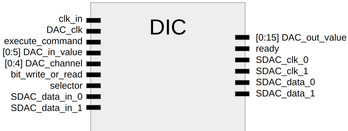
Figure 4.23: The DIC module input/output ports. Interfaces with the ABACUS chip and requires a 100 MHz clock via the clk port for FSM synchronization. The DAC_clk port, using a 100, kHz clock, handles the ABACUS serial CLK. The execute_command port initiates the command execution, generating a payload based on [0:5] DAC_in_value as the DAC value and [0:4] DAC_channel as the channel address. The bit_write_or_read input dictates whether to read (0b0) or write (0b1) data. One DIC module can manage two ABACUS chips, and the selector input determines whether to communicate with the even-labeled (0b0) or odd-labeled (0b1) ABACUS. The ready output flag allows users to monitor the module’s status. For read commands, the full 16-bit output in the form of Table 4.2 is mapped to the DAC_out_value bus. Ports directly connected to the ABACUS are: two clock ports ( SDAC_clk_0 and SDAC_clk_1 ), two data ports ( SDAC_data_0 and SDAC_data_1 ), and two input ports ( SDAC_data_in_0 and SDAC_data_in_1 ). These ports handle the CLK, SIN, and SOUT signals of the even (port name ending with 0) or odd (port name ending with 1) ABACUS, respectively.
