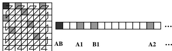
Fig. 3 Zig-zag scan and odd/even split of the DCT coefficients. The black position is the DC, while the grey ones represent the non-null AC coefficients.
