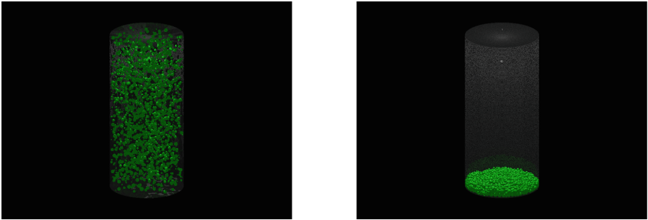
Fig. 1. Initial (left) and final (right) configuration generated in a simulation of the agglomeration process of a multidisperse system of 2,000 spherical particles in a cylinder.
