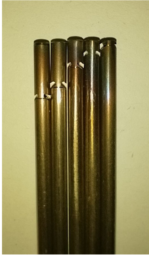
Figure 2.4: Tubes for ethylene input downwards under the cathode. From left to right, the slits depth is 10, 8, 5, 3 and 1 mm.
