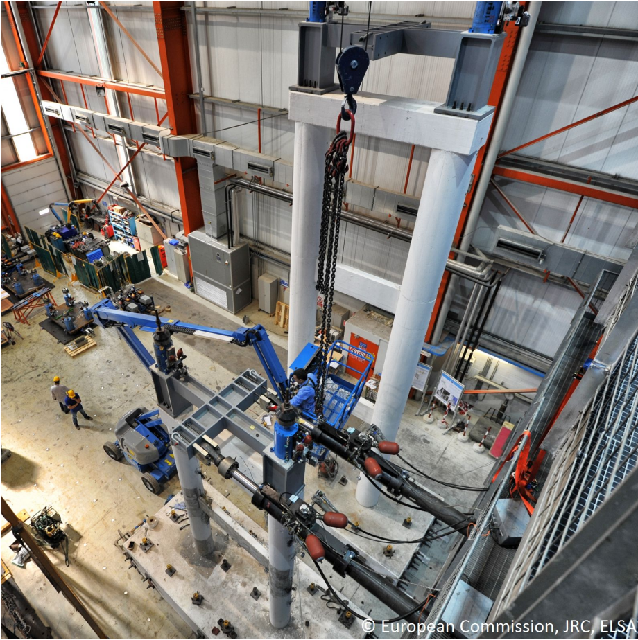
Figure 4.5: Mock-up 1:2.5 scale specimens of Piers #9 and #11
