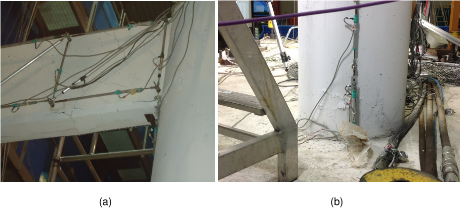
Figure 4.34: Close-up views of Pier #11: a transverse beam and b left column, after Test k09, i.e. non isolated bridge at ULS.
