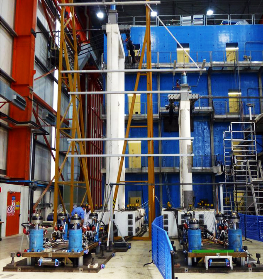
Figure 4.11: Mock-up 1:2.5 scale specimens of Piers #9 and #11 with relevant FPB isolator pairs
