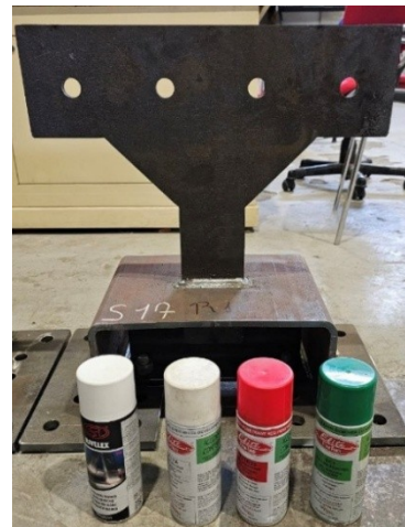
(b) Spray penetrant testing
