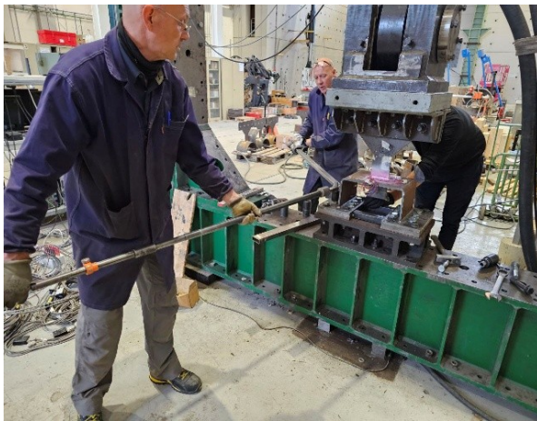
(a) Pre-tensioning of the bottom connection to the frame
