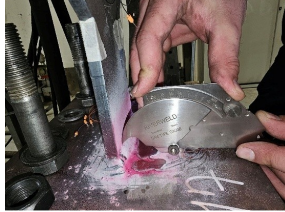
(b) Measuring the actual throat thickness of the RHS-LCT-FSW joint
