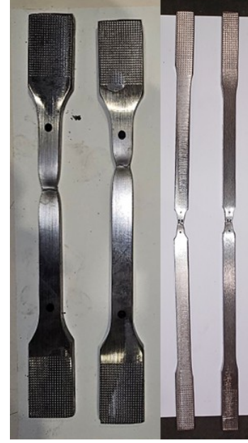
(b) Fractured coupon specimens.
