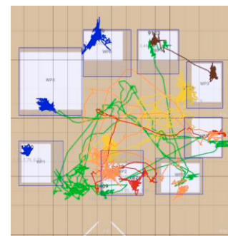
Fig. 3: RTLS based spaghetti diagram
