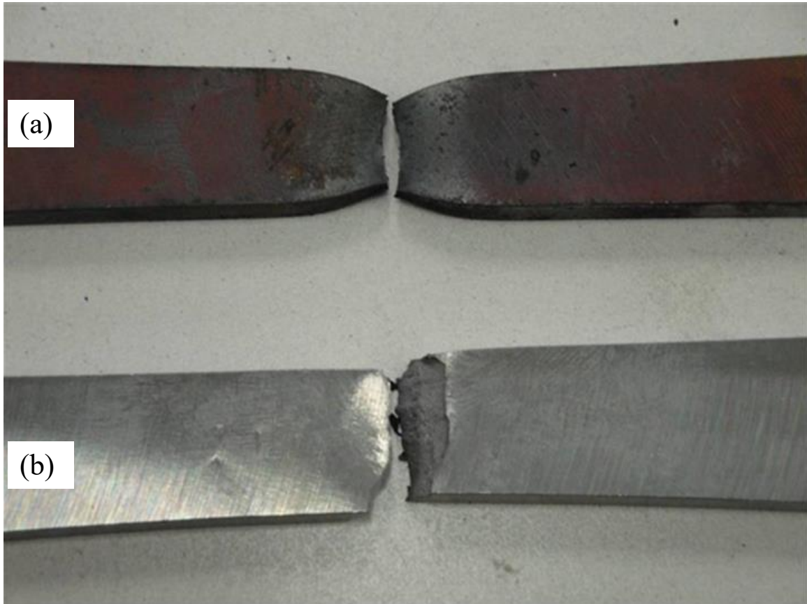
Figure 8. Fracture surface of plain specimen tested at 650°C (a) ( \Delta\sigma=140 MPa, N=284049 ), and room temperature (b) ( \Delta\sigma=900 , N=155000 )
