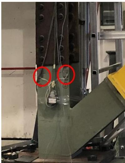
Figure 4 - Base column instrumentation: strain gauges
