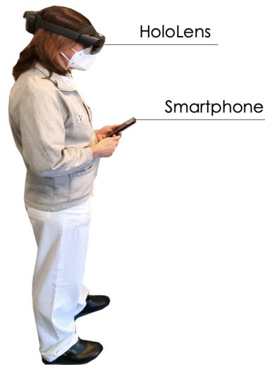
Figure 1.16: Example of combined use of HoloLens and a smartphone to simplify interaction with virtual cues.
