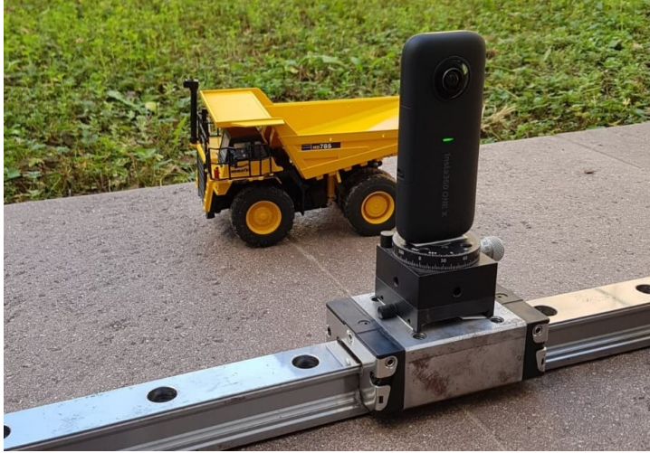
Figure 3.22: Experimental setup to test the developed algorithm. A 360° camera is placed on a rotary and a translation stage. The camera frames the miniature model of a truck.
