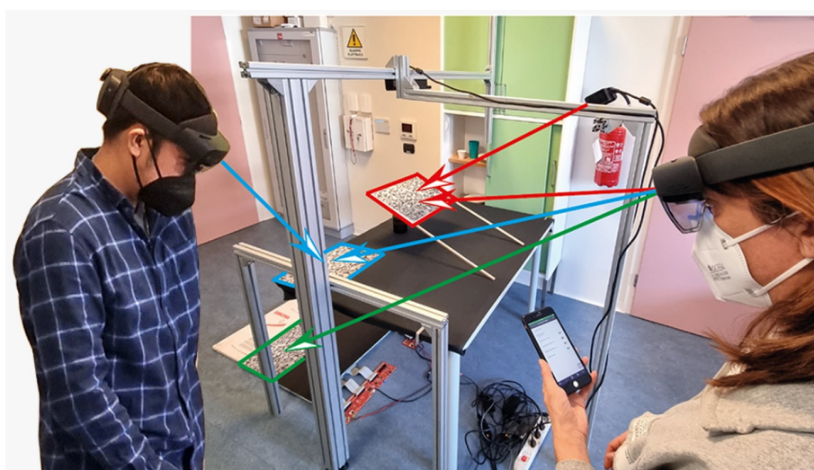
Figure 2.12: Spatial Anchors setting: the red image target is used by the therapist's HoloLens and the Kinect to operate in the same reference system; the blue target is used by the therapist's and the patient's HoloLens to have the same reference system of the working plane; the green target is used only by the therapist's HoloLens to localize the baropodometric platform in space.
