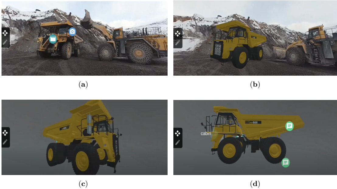
Figure 3.15: Transitioning from 2D video to the 3D virtual object: (a) 2D video. (b) Object replacement after detection and localization. (c) Object rotating in front of the user’s viewpoint. (d) Digital information contextualized with the vehicle model. The corresponding videos can be found here.
