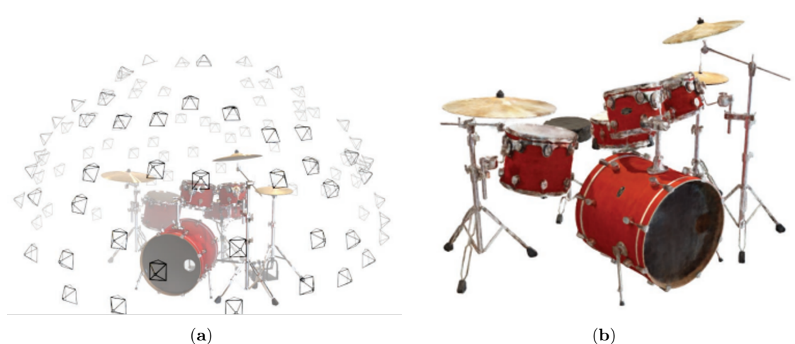
Figure 3.13: NeRF input as a set of calibrated images (a) and output a 3D scene representation (b). © from [73].
