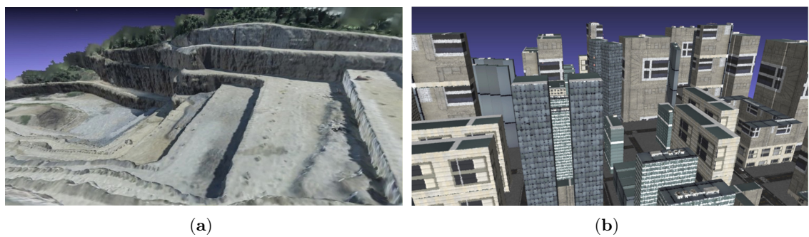
Figure 3.12: Final results after the 3D reconstruction for the mine (a) and the city (b) environments.
