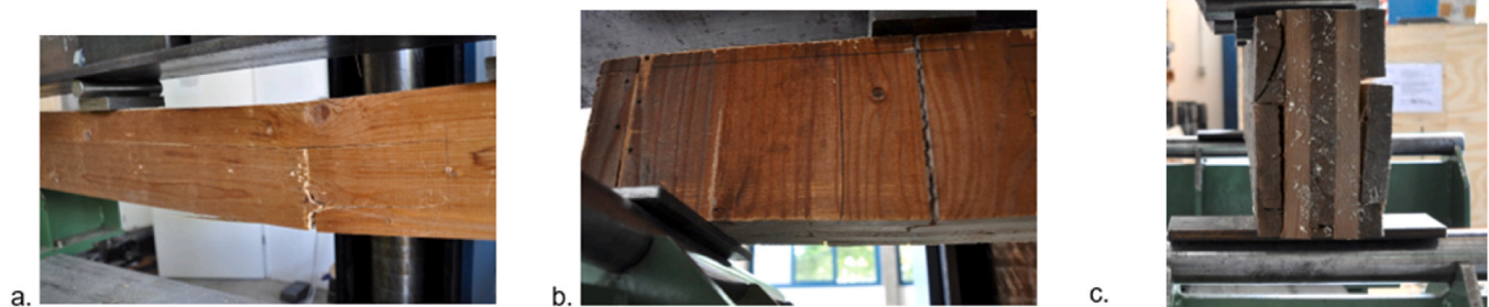
Fig. 8. CLT beam failure mode: a) bending, b) net shear, c) torsional shear.
