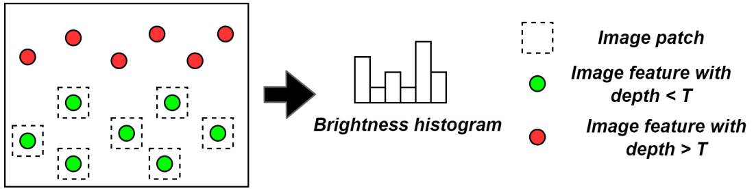
Figure 4.7: Representation of the proposed camera exposure control.
