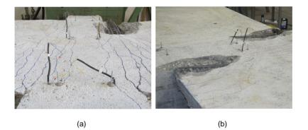
Figure 7.11: Damaged specimen after (a) SQ1C, and (b) SQ2C cyclic tests
