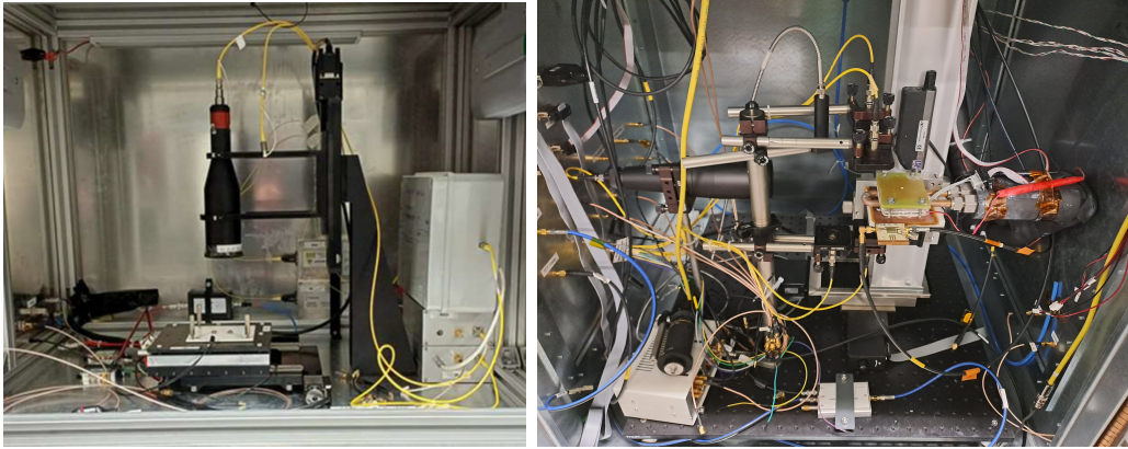
Figure 4.3: Setups used for the measurements of the samples. Left - Faraday cage that hosts the Large Scanning Transient Current Technique (TCT) setup in FBK laboratories. On the right side of the picture, the box that allows for splitting the laser pulse into two is visible after the beam monitor. Right - Inside the Faraday cage where the TCT- setup at CERN is located. Linear stages and the optical system are visible along with the amplifier at the bottom of the setup. The Peltier cell and the cables for cooling are on the right, connected to the sample.
