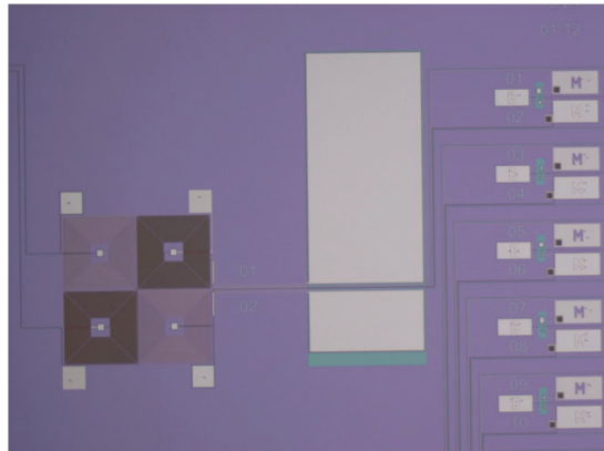
Figure 5.2: Two LC filters. On the left two pairs of spirals for two inductors are shown, on the right two capacitors (white) differently shaped to reach different capacitances. On the far right, bonding pads are visible.
