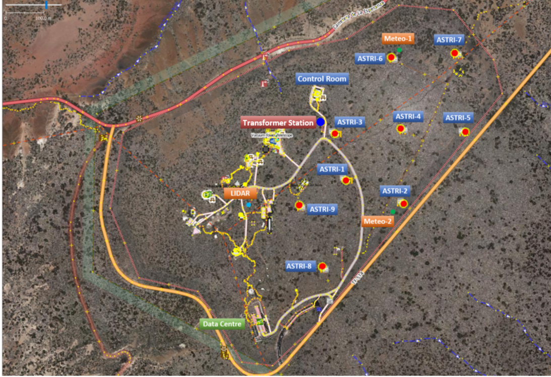
Figure 2.5: Final layout for the ASTRI Mini-Array at the Teide Observatory, from [38]. The Figure shows the final positions for the 9 telescopes, the position of the two meteorological towers, the position of the LIDAR, the position of the transformer station and that of the local control room and of the data centre.
