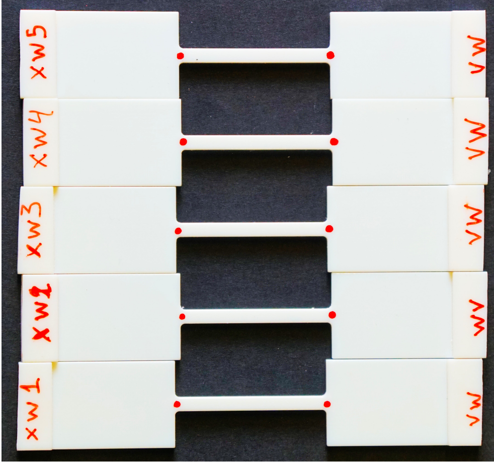
Figure 1.18. The fabricated dog-bone samples uni-axially tested to estimate the mechanical properties of the bulk material (Vero PureWhite™) used to print the FG lattice structures.
