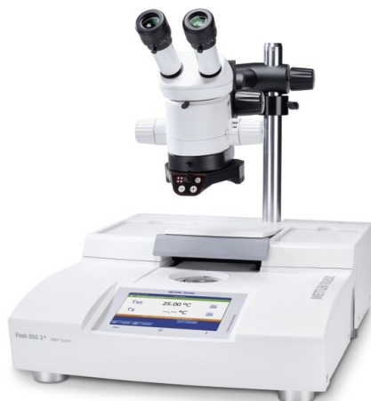
Figure 3.36: Photograph of the Mettler-Toledo Flash DSC 2+ instrument used for fast scanning calorimetry measurements [227].
