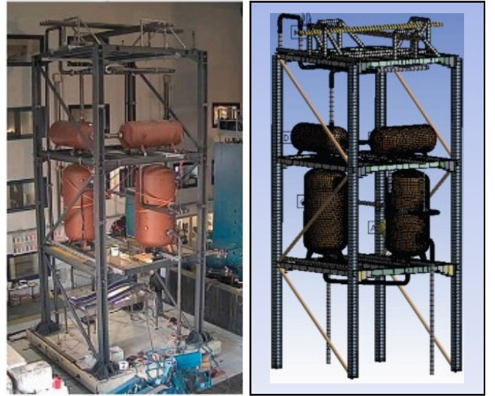
FIGURE 2: (a) Photo of the lateral view of the SPIF mock-up; (b) refined FE model.
