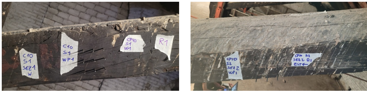
Figure 2. Woodpecker and Resistograph tests on the same cross-section.
