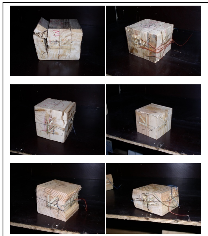
Figure 5. Combined diagram of elastic anisotropy of wood (a) and the nature of sample destruction (b)
