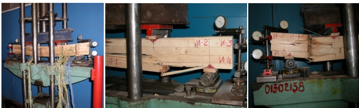
a) beams under load and at the moment of destruction
