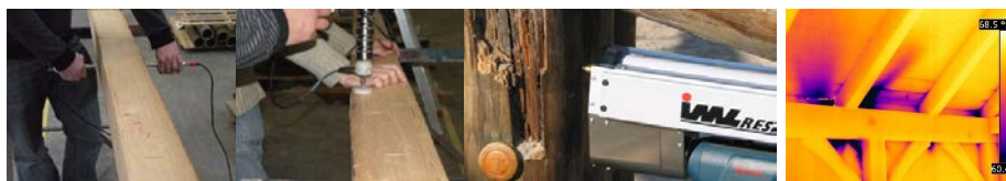
Figure 1. Different NDT methods: ultrasound, moisture content measurement, drill resistance, infrared thermography
