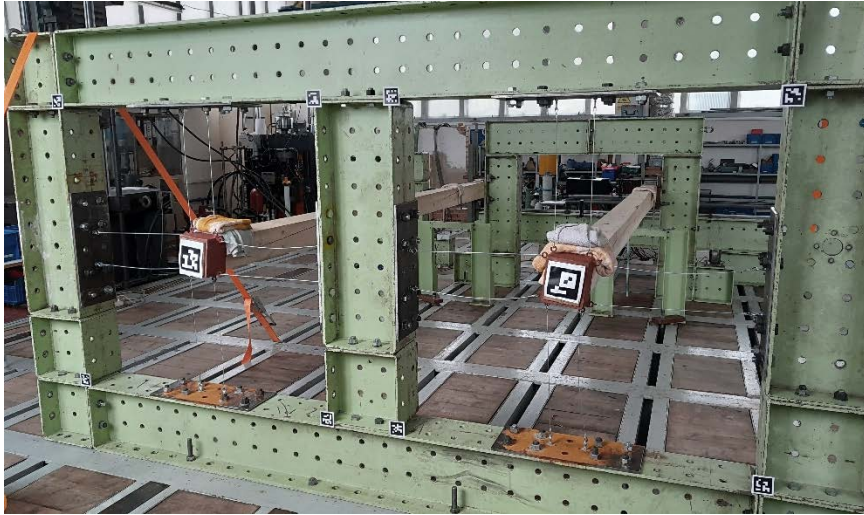
Figure 1. Beams in the testing hall equipped with ArUco markers [6] for precise displacement monitoring.
