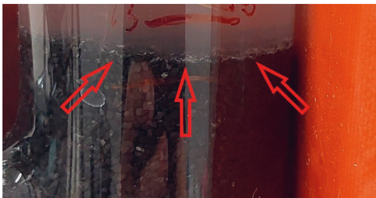
Figure S12. Picture of whitish substance spotted on the granular activated carbon (GAC) bed in the heterotrophic fluidized bed bioreactor during PHASE IV+FC that could possibly represent elemental sulphur.
