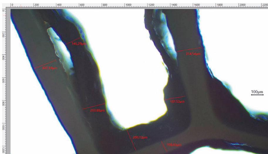
Figure S8. Particular of biofilm detachment from K5-MBBR carrier (optical microscope, 40x magnification) at salinity 7.5%. Approximately, one fourth of the total biofilm detached from the carrier by a visual estimation.
