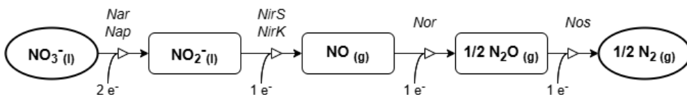
Figure 1. Denitrification reductive steps from nitrate to nitrogen gas and the enzymes involved. Nar and Nap: nitrate reductases, NirS and NirK: nitrite reductases, Nor: nitric oxide reductase, Nos: nitrous oxide reductase. Modified from Di Capua et al. (2019).
