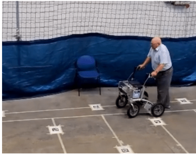
Figure 4.1: The FriWalk robotic rollator using adaptive shared control paradigms with an elderly person.
