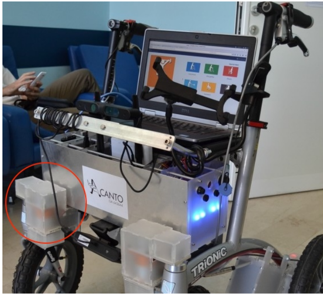
Figure 2.2: The FriWalk robot. The red circle highlights the DC motors mounted on the front wheels and their encoders.
