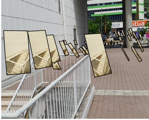
Figure 4.11: Acquisition process: images are collected through the smartphone coupled with the RTK-GNSS receiver, and positioned in the environment, according to their camera pose.
