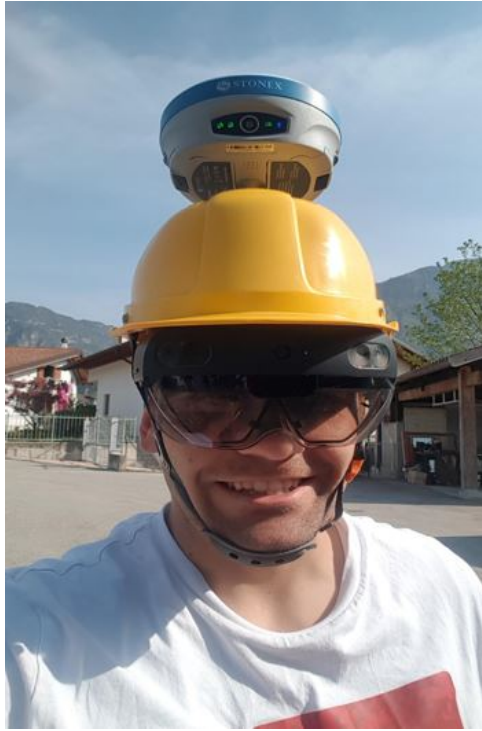
Figure 4.16: The helmet as a support for the combination of the Stonex and the HoloLens
