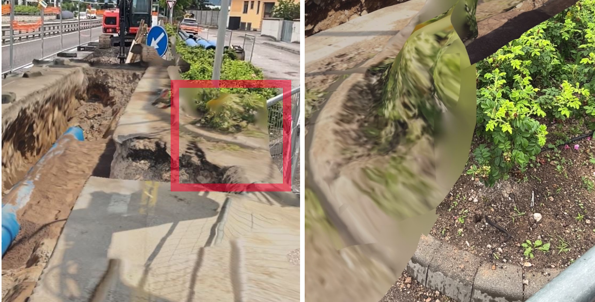
Figure 4.13: (left) A scenario is shown, where the real scene is over-imposed with the virtual (pre-acquired) counterpart. Here, the specific case study is the excavation. The zoom of the red square area is also shown (right). The spatial accuracy of the over-imposition is very good.
