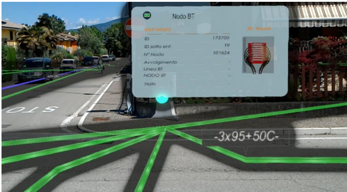
Figure 4.17: The visualization of the holograms of the underground net from the Hololens
