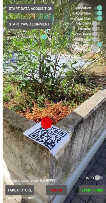
Figure 4.9: Error measurement process: the QR code top-left finder pattern is placed on the acquired spot, and the red holograms are placed using the acquired GCS pose.
