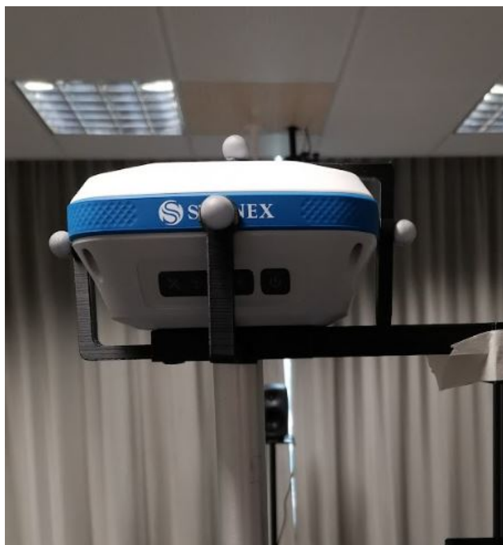
Figure 4.3: Custom 3D printed structure for the creation of the rigid body of the RTK-GNSS device within the MoCap reference system.
