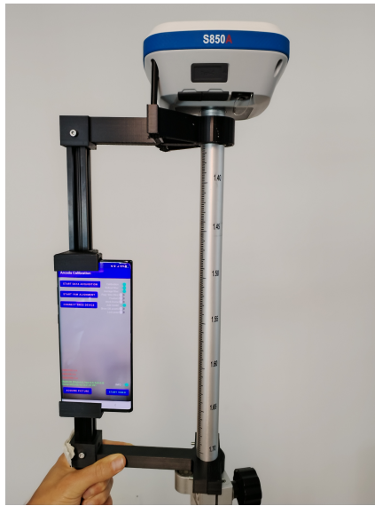
Figure 5.2: System acquisition composed by Stonex and Smartphone for obtaining high accuracy georeferenced images
