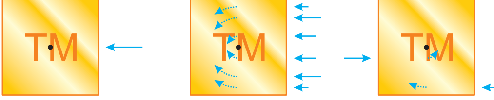
Figure 3.5 – The scheme, that represent the 1-TM torsion pendulum see from above (the black dot in the center of the TM is the torsional fiber, entering the page), shows some example of force combinations that would be invisible to this facility, but dangerous on a really free TM in space. While the right hand example, where the torques induced by two completely asymmetric forces exactly cancels out because of different arms, is quite improbable given the symmetry of the GRS, the other two cannot, for the same reason, be excluded and need investigation.
