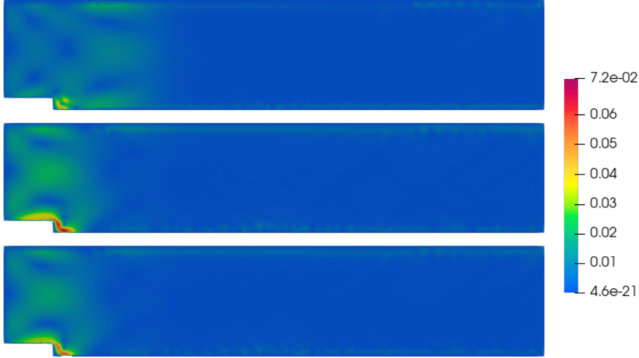
Figure 3.13: Pointwise difference between AD applied to G-ROM and G-ROM, r = 10 , \delta = 0.6 and . 1 st : Lavrentiev with \mu = 0.1 ; 2 nd : Tikhonov with \mu = 0.1 ; 3 rd : van Cittert with N = 10 .
