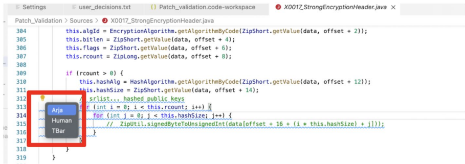
Fig. 2 View of the plug-in used by the participants. This an example of the view of the participants when using the plug-in into VS Code. The plug-in shows the identified faulty line and it shows the proposed the patches for that specific vulnerability
