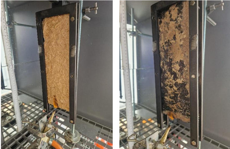
Figure 4.9 Representative images during the single flame source test of TSCs samples: (a) CA60 (based on xanthan gum) and (b) ID5 (based on gelatin).
