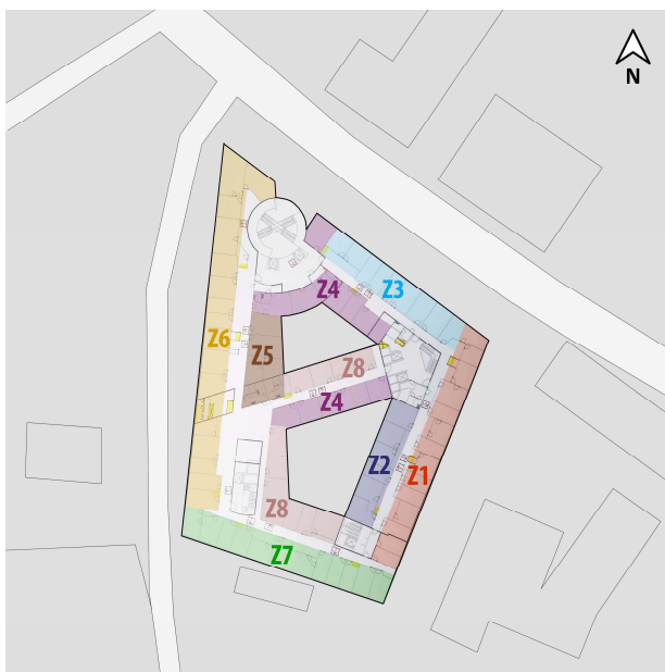
Fig. 2. Distribution of the HVAC zones.
