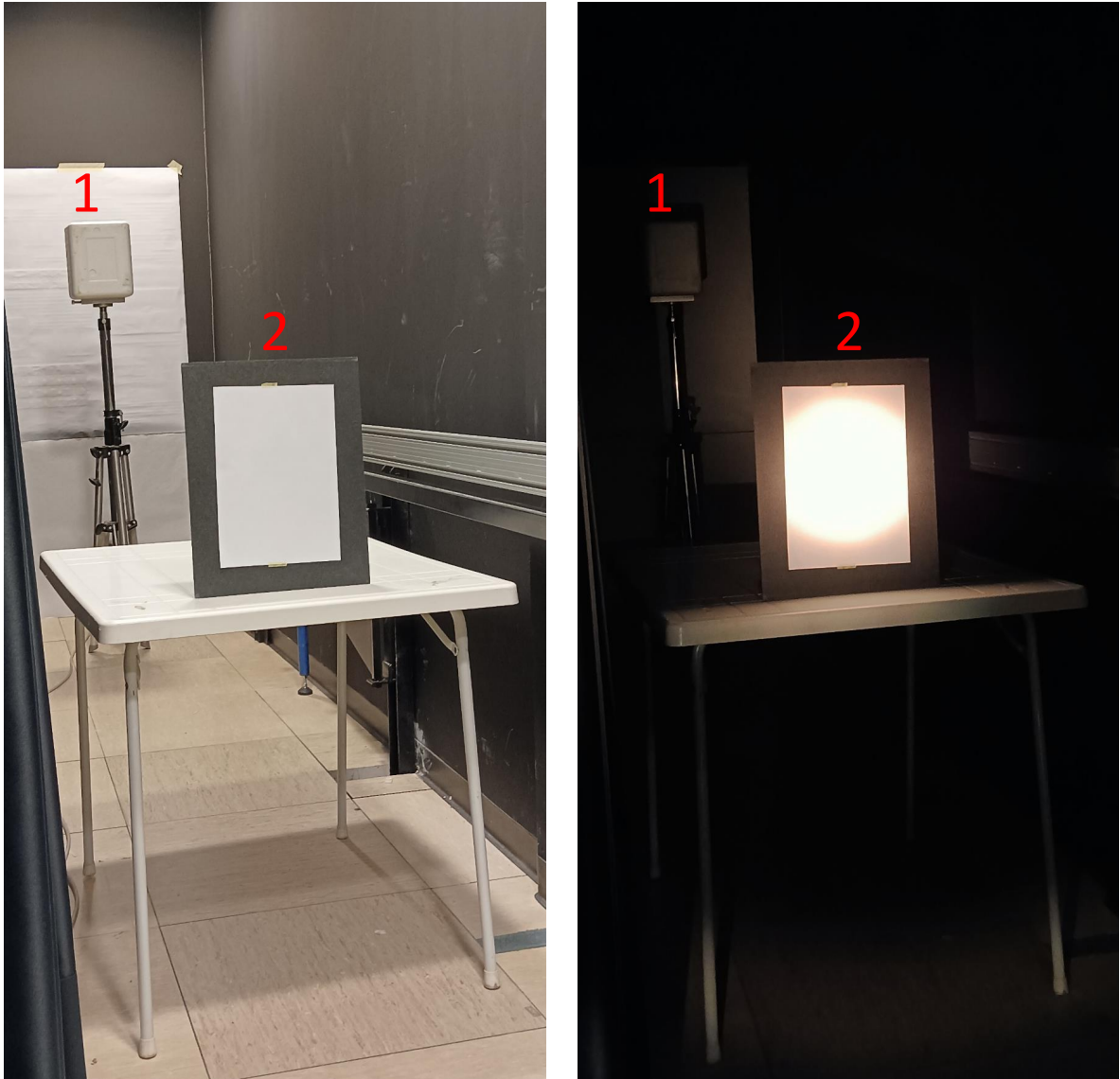
Figure 4.8: Laboratory setup for the qualitative evaluation of AS and coincidence techniques. Target nr. 2 was illuminated by a collimated fiber optics halogen lamp, emulating a highly reflective target reflecting an intense background illumination. In order to place the system close to a realistic scenario, the optical bandpass filter was removed.
