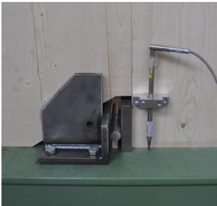
Figure 10: Shear blocks and steel rod (a); steel plate and steel bar for load transfer to each panel (b).
