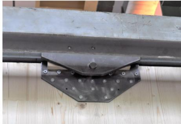
Figure 10: Shear blocks and steel rod (a); steel plate and steel bar for load transfer to each panel (b).
