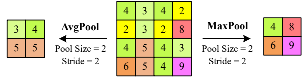
Fig. 3. The illustration of an example of the AvgPool and MaxPool operations.
