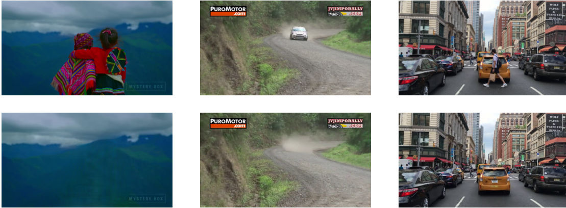
Figure 4.3: Original frames (first row) sampled from videos in our dataset and the corresponding inpainted frames (second row) obtained using STTN. In the inpainted frames, specific regions of the frame have been replaced spatio-temporally coherently with respect to the current and neighboring frames.
