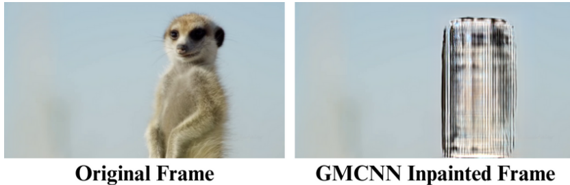
Figure 4.12: Problems related to GMCNN when used to inpaint large objects in video frames.
