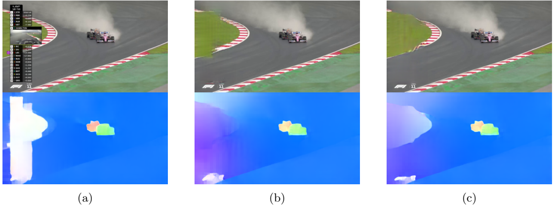
Figure 4.6: Dense Optical Flow Field estimated using RAFT [106]. Sub-figure (a) shows the dense optical flow field estimated from frames of a real video \mathbf{C} . In contrast, sub-figures (b) and (c) show, respectively, the dense optical flow fields estimated on inpainted video frames \mathbf{IVF} produced with OPN and STTN. Note that in (b) and (c), it is possible to notice “distortions” in the color gradient in correspondence to the inpainted region, while in (a), this does not happen, except for the presence of the race ranking.
