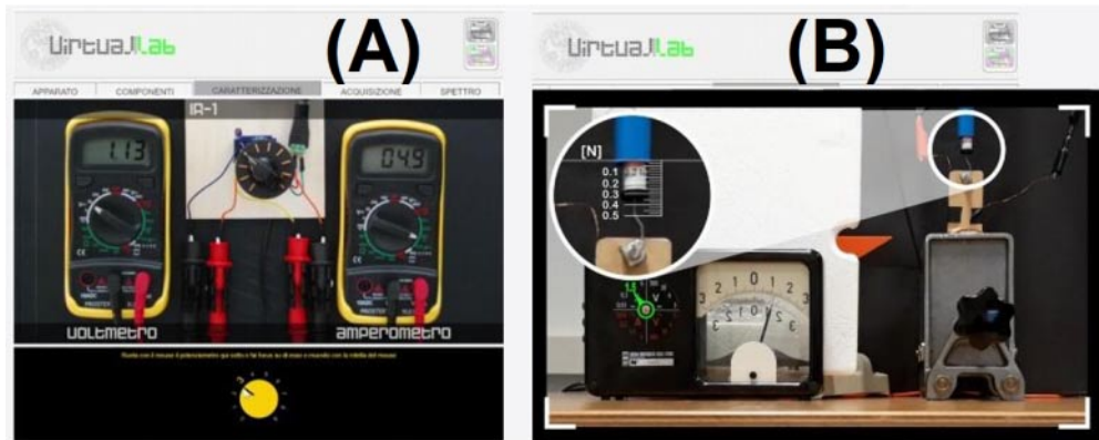
Fig. 7. – Two VRLs designed by a member of our group. (A) The measure of Current vs. Voltage curve for a LED. (B) The force on a current carrying wire.
