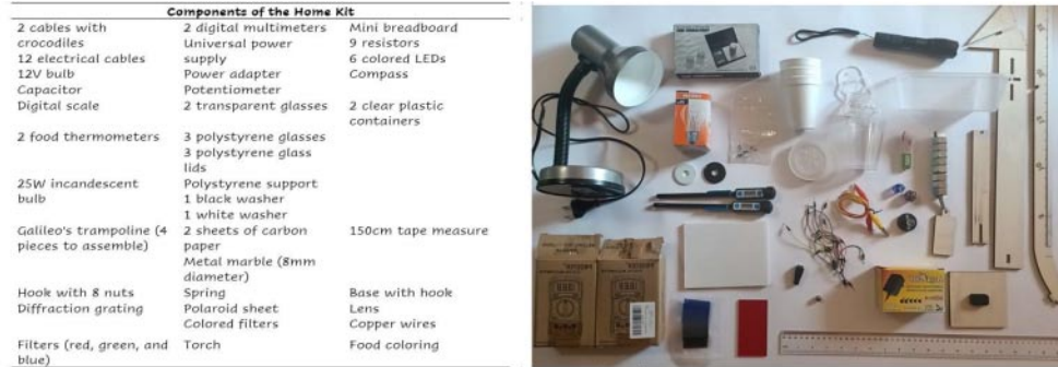
Fig. 3. – Summary table and components of the home-kit provided to the students.
