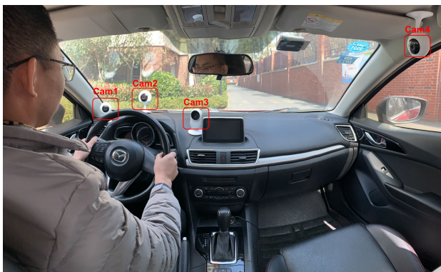
Fig. 4. The camera locations in the 100-Driver dataset. Cam1: front-left, Cam2: front, Cam3: front-right, and Cam4: side-right.
