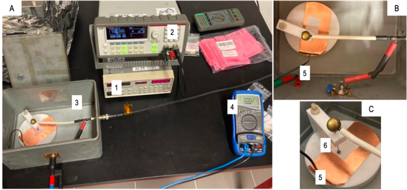
Figure 21 The setup for dielectric breakdown measurements is here reported. In Figure A: 5 kV HV source (1), Keithley oscilloscope (2), testing box (3), digital multimeter (4). In Figures B and C: plastic frame for the testing with the grounded bottom copper electrode (5) and the spherical top electrode (6) connected to the HV source.
