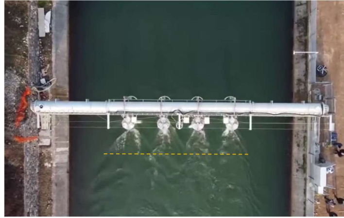
Fig. 5-6. Near-wake distribution of four cross-flow turbines from [4].
