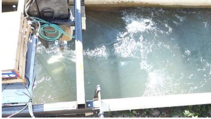
Fig. 4-8. Top-view of the canal during high-speed turbine operation.
