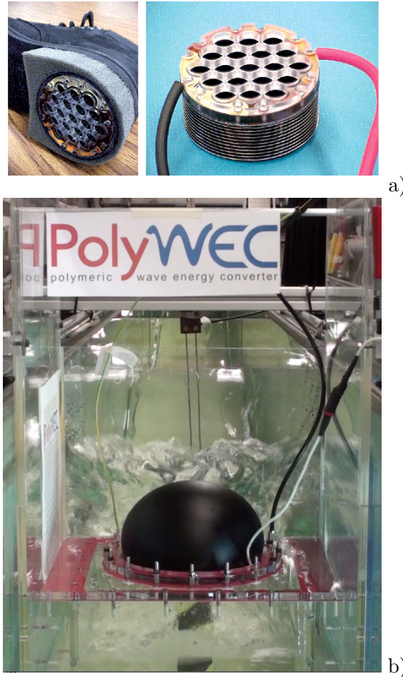
FIGURE 1.1: Examples of DE energy harvesters: a) heel-strike generator tested by SRI international [10] and b) polymeric oscillating water column developed in the PolyWEC project [61].
