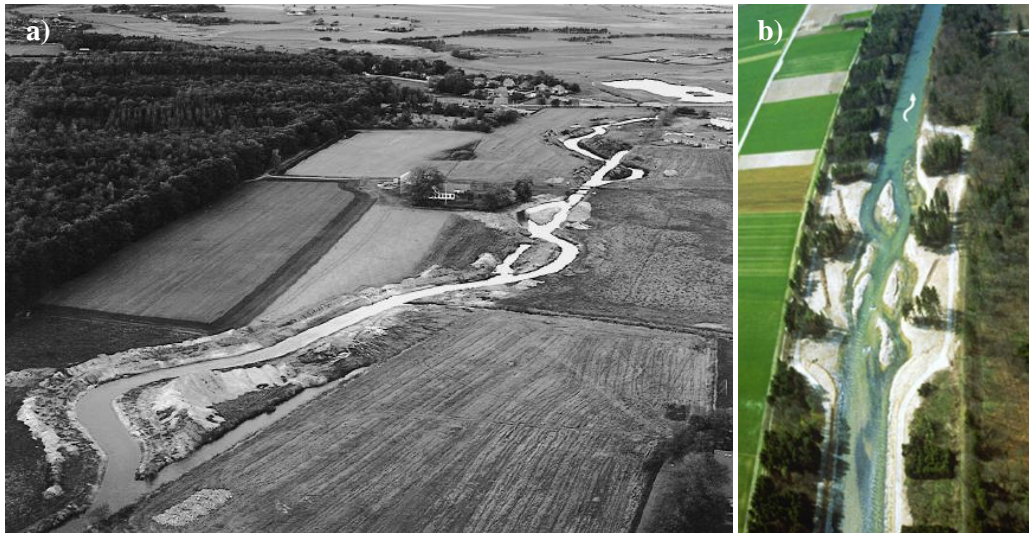
Figure 1. Images showing examples of river restoration projects a) re-meandering of the straightened reach of River Brede at Logumkloster, Denmark and b) local widening along the straight reach of River Emme at Aeflingen, Switzerland (Courtesy: Dr. Alessandra Crosato)
