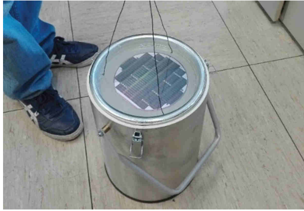
FIGURE 4.1: Manual immersion of a SiPM wafer in dewar filled of liquid nitrogen
