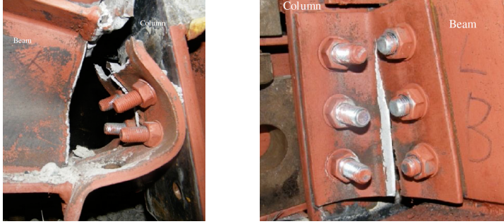
Figure 2.8: Failure modes of the specimens (Yang and Tan [2013b])
