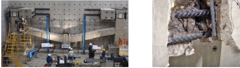
Figure 2.9: Failure modes of the steel and concrete assemblies (Sadek et al. [2011])
