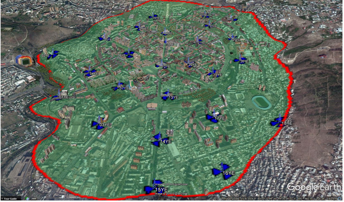
Figure 6.1 – An operational LTE-A network with 26 eNBs (in total 209 cells) in the city center of Yerevan. Each eNBs is composed of variable number of sectors, which in turn is composed of variable number of carriers employing 20MHz, 15MHz and 10MHz LTE channels.
