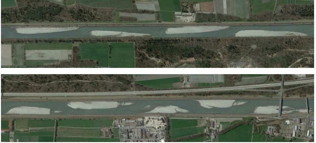
Figure 4.8: Two different reaches with alternate bars in the Alpine Rhine river. The upper one shows alternate bars of the upstream reach of Figure 4.6 ( Source: "Alpine Rhine"; 47°1'58.75"N, 9°29'32.43"E. Google Earth. February 04, 2012. January 7, 2016) the lower one refers to the central part of the reach ( Source: "Alpine Rhine"; 47°7'10.92"N, 9°30'54.28"E. Google Earth. February 04, 2012. January 7, 2016). Different bar wavelengths and different shapes are visible from the aerial images. Water flows from left to right, width of the river is around 95 m in both the images.
