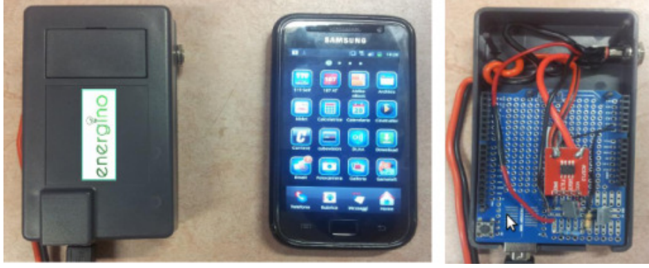
Figure 3.2: Energino : Hardware and software solution for power consumption monitoring
