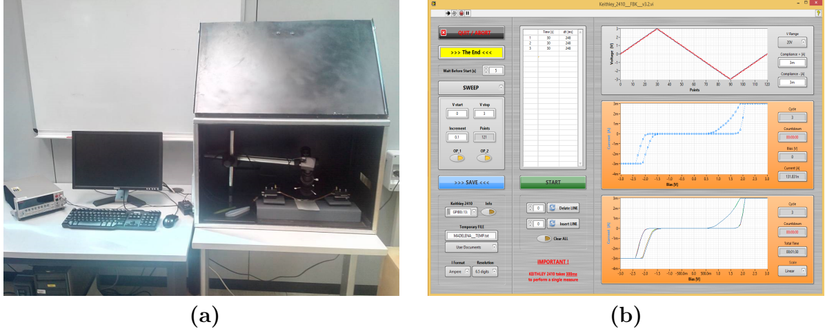
FIGURE 2.8: Inorganic memristor measurement and data acquisition setup. (a) , Measurement setup composed by a Faraday cage, stereoscopic microscope, micro-manipulators with tungsten tips or Platinum wire, 2410 Keithley High Voltage Source Meter. (b) , LabVIEW data acquisition control panel of program for inorganic memristive device testing
