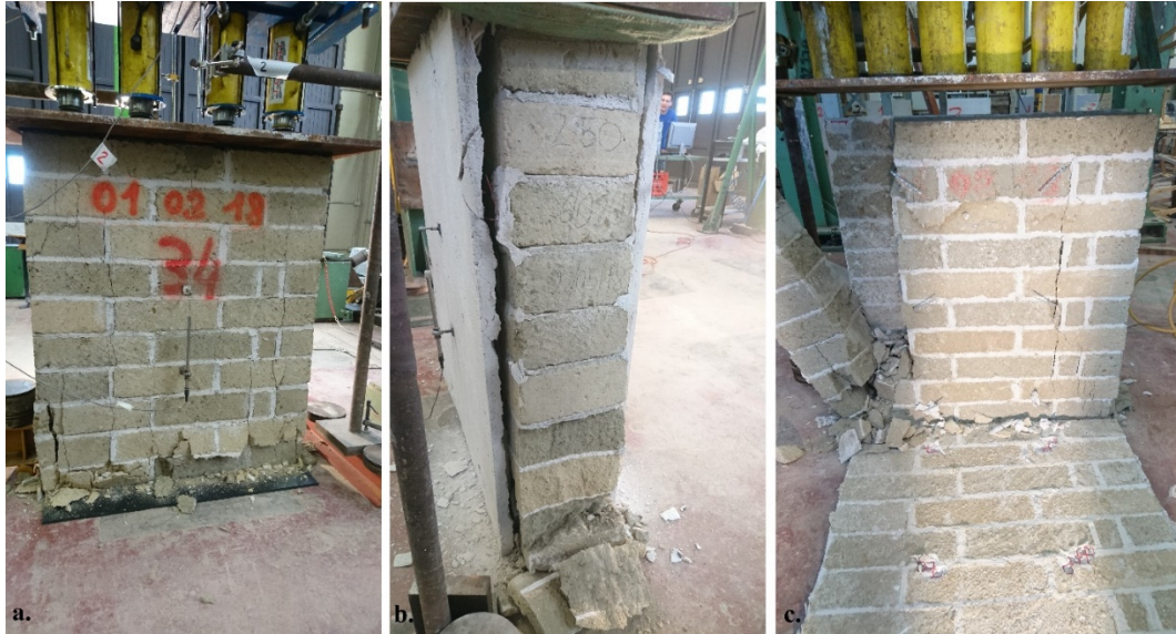
Fig. 8 – Failure modes of the unstrengthened (a) and strengthened (b,c) tuff masonry walls.
