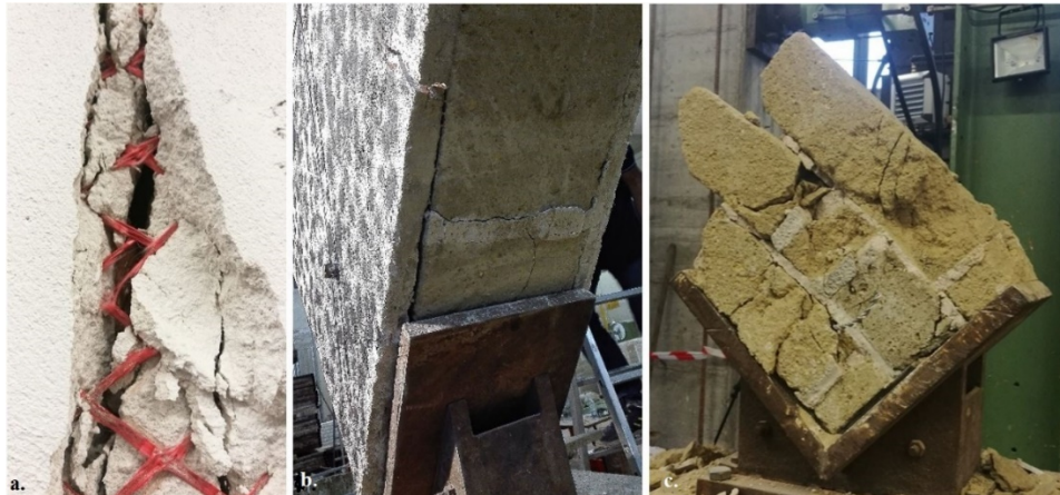
Fig. 13 – Details of the failure modes observed: (a) fabric failure, (b) detachment of the TRM curtains (tuff panels), (c) masonry crushing (tuff panels).
