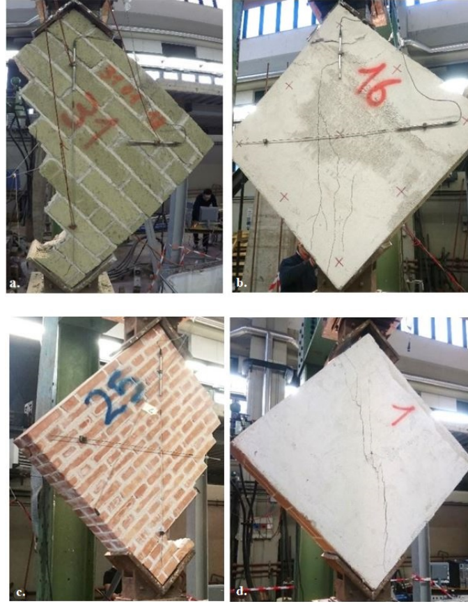
Fig. 12 – Failure modes of tuff and fired clay brick masonry panels: (a) tuff unreinforced; (b) tuff reinforced with TRM; (c) fired clay brick unreinforced; (d) fired clay brick reinforced with TRM.
