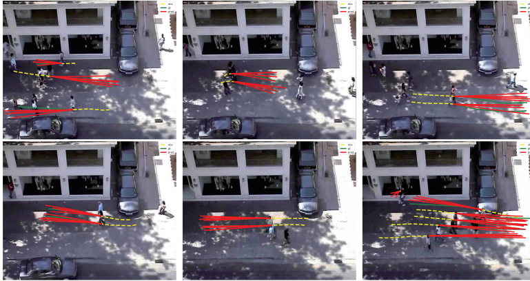
Figure 11: Visualizations of the prediction performances on the zara1 and zara2 subsets. The dash line indicates the observation sequence, the red solid line indicates the prediction sequence, and the green solid line corresponds to the ground truth.
