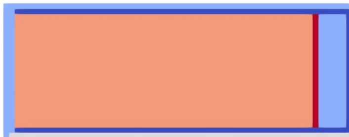
Figure 2.64: Container with a dielectric false bottom filled with tobacco.
