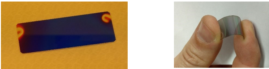
Figure 2.9. Fabricated samples. The multilayer films deposited on a silica substrate (left); the multilayer films deposited on a flexible polyester substrate under bending (right).
