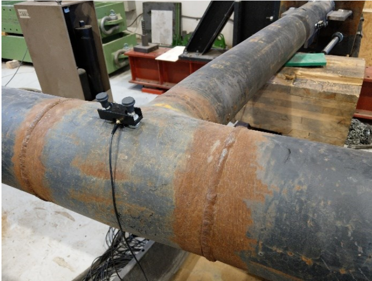
Figure 3.16 Acoustic sensor installation on the Tee joint. Typical MAG4M magnetic spring clips used to attach the VS150 sensor on the pipeline.
