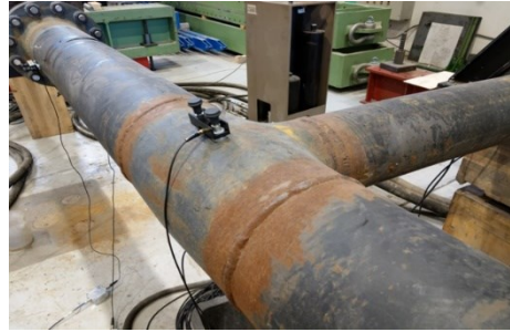
Figure 3.19 Green points show acoustic emission signals detected on the Tee joint during the HS tests (left). Tee joint component (right).
