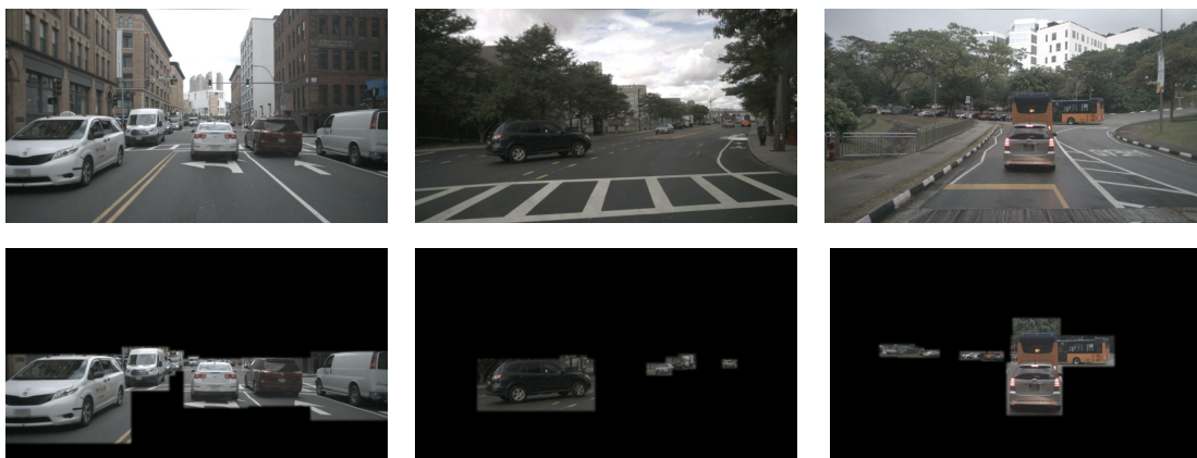
Figure 8.3: Examples of the attention mechanism applied in three different scenarios: the first row shows the original images, and the second row displays the results of “paying attention” to the vehicles.
