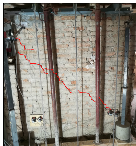
Figure 10. Specimen 2 as-built (AsB-2): (a) load–displacement curves; (b) crack pattern at peak loading
