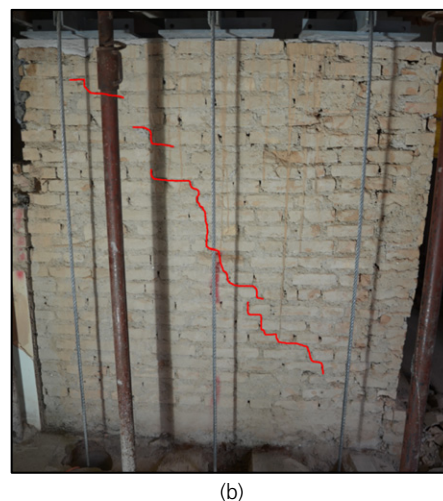
Figure 6. Specimen 1 as-built (AsB-1): (a) load–displacement curves; (b) crack pattern at peak loading
